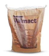
Use: It is a grounding intensifier material specially designed to reduce the electrical resistance of groundings, made up of 2 components, A and B. Component A is a high electrical conductivity material, and Component B allows greater compaction and bonds it to the electrode, ensuring close contact, which results in lower resistance.
