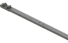
Uso: Supports conductors and equipment in Medium Voltage overhead lines Material: Tubular profile PTR of 101.6 mm x 51 mm C14
