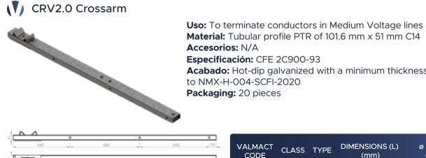
Especificación: CFE 2C900-93 Acabado: Hot-dip galvanized with a minimum thickness of 70 µm according to NMX-H-004-SCFI-2020 Packaging: 20 pieces CLASS TYPE DIMENSIONS (L) **APPROXIMATE** ø HOLES WEIGHT (KG)
